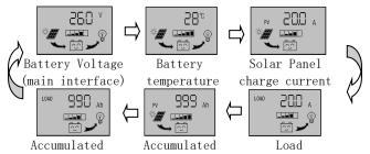
Discharging power (Ah) charging power (Ah) discharge current
