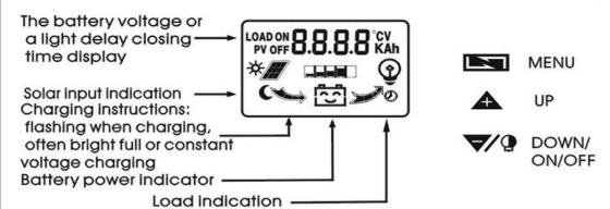
MENU: switch between different display, or to enter/exit setting ty long press.
