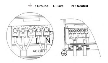
**Note:** The grounding wire shall be as thick as possible (cross-sectional area is not less than 4mm2). The grounding point shall be as close as possible to the all-in-one solar charge inverter. The shorter the grounding wire, the better.
