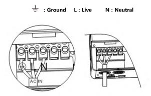
③ Properly connect the AC output wire according to the wire sequence and terminal position shown in the figure below. Please connect the ground wire first, and then the live wire and the neutral wire. The ground wire is connected to the grounding screw hole on the cabinet through the O-type terminal.
