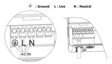
③ Properly connect the AC output wire according to the wire sequence and terminal position shown in the figure below. Please connect the ground wire first, and then the live wire and the neutral wire. The ground wire is connected to the grounding screw hole on the cabinet through the O-type terminal.
